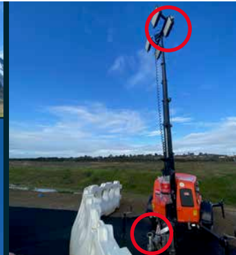
3. Mast must be lowered to tow.
